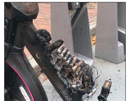
Faulty battery sends an e-scooter up in flames
